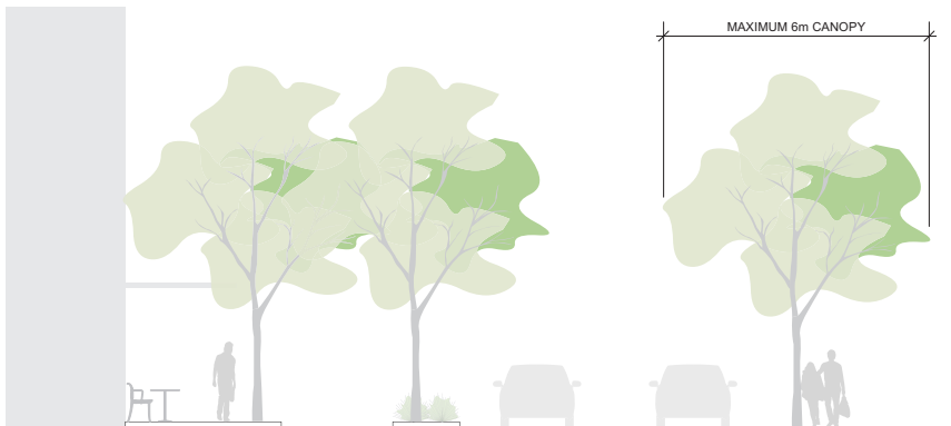
INDICATIVE SECTION OF TREES PLANTED UNDER POWERLINES
