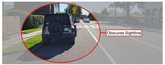
Figure 8.7: Parked Vehicle near the Raised Pedestrian Crossing along Gale Street
