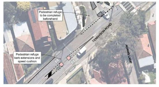
Figure 9.4: Pedestrian Refuges and Speed Cushions – Tennyson Road
