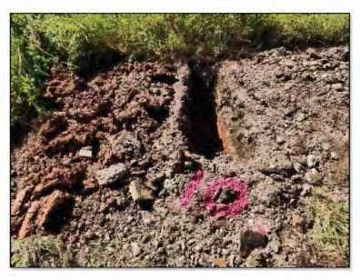
**Photo 11**Test Pit TP10 where one of the Asbestos hotspots was discovered
