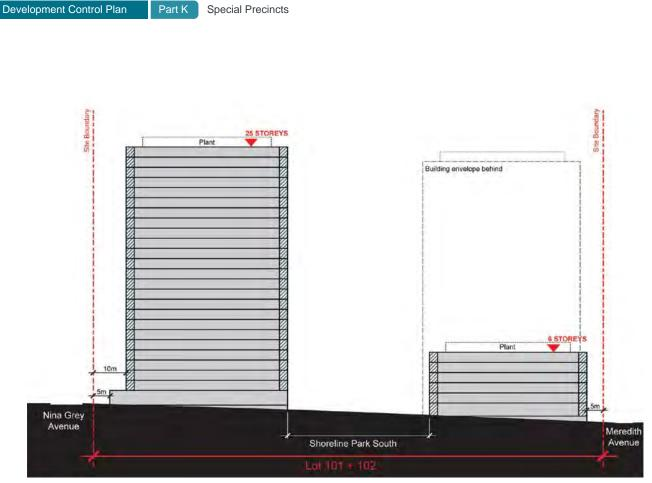
Figure K17-22 Precinct C Building Envelope Section A-A
