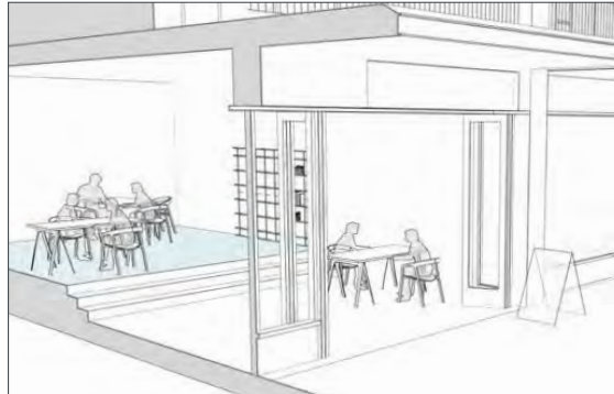
Building entry at street with internal steps/ ramp/ retractable stair/ lift system to elevated floor above flood level
